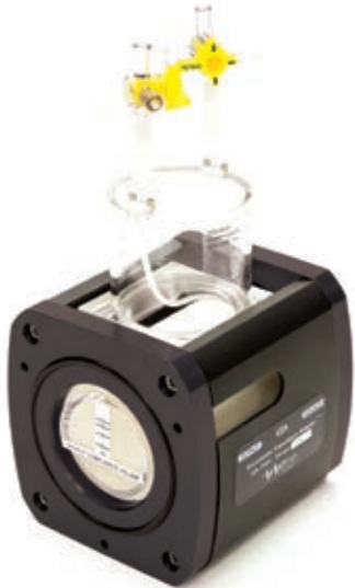
A Viscoelastic Impedance Adaptor provides input waveform compliance to create physiological pressures and flows.
