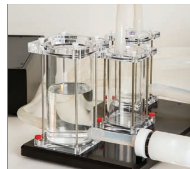
A compliance assembly provides adjustable air volume to allow system tuning for a wide range of pressure conditions.
