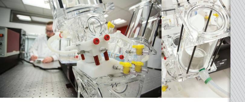
The Pulse Duplicator System assesses the performance of cardiovascular devices and prosthetic heart valves under simulated cardiac conditions. It simulates physiological or other complex flow variations while allowing the user to vary the peripheral resistance and compliance of the system. Pressure ports and flow measuring locations allow for data to be collected from aortic or mitral sites. Transparent viewpoints allow multiple viewing angles of the valve including inflow and outflow.
