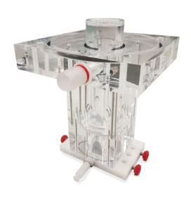
The PIV Load Assembly provides an optically clear, anatomically representative aortic inflow and outflow to enable Particle Imaging Velocimetry studies in the Pulse Duplicator. The PIV Load Assembly replaces the lower half of the standard aortic load assembly and is easily substituted into the ViVitro Labs Pulse Duplicator.
