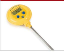
A digital thermometer allows easy fluid temperature measurement in the Pulse Duplicator.
