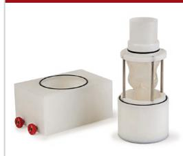
The ViVitro Aortic Conduit Mount (ACM), formerly the Left Ventricular Outflow Tract (LVOT), is used to mount a compliant conduit, native or synthetic root, and test percutaneous valves in the ViVitro Model Left Heart system.
