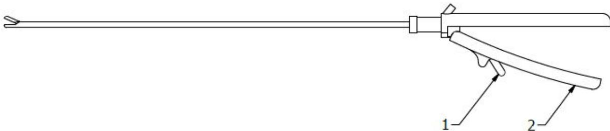
Drawing No. 11. Laparoscopic needle holder diagram (1 – needle release button, 2 – handle)
