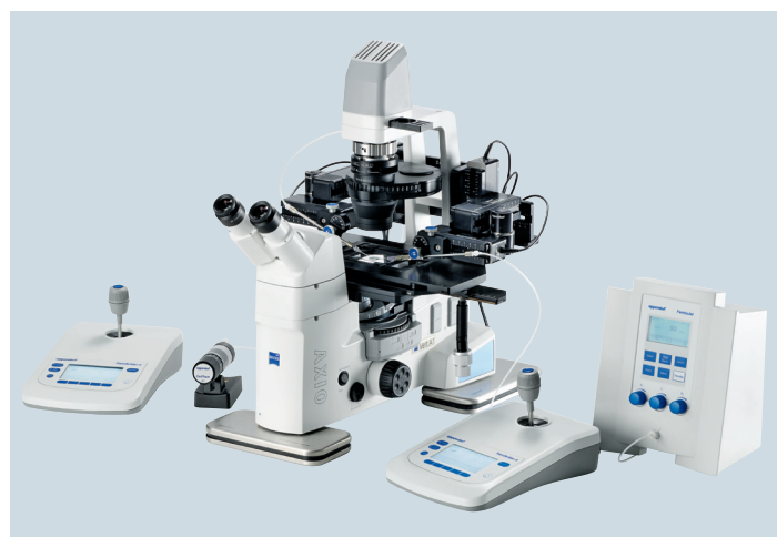
Fig. 4: Workstation set-up for microinjection of nucleic acids into the zygote: TransferMan 4r, CellTram Air and FemtoJet in combination with Zeiss® Axio Vert.A1 microscope.
